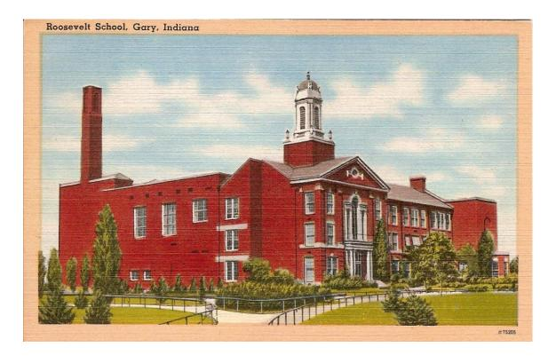
The original Roosevelt school (pictured above) was completed by 1930 with a 1946 addition that balanced the façade with a west wing and new gymnasium to the rear. This three-story, historic core is built on a reinforced concrete foundation and steel superstructure, comprised of red and brown brick with classical flourishes of limestone. Echoing the collegial aesthetics of Gary's other public schools, Roosevelt was set back from the street and featured a grand front lawn.
